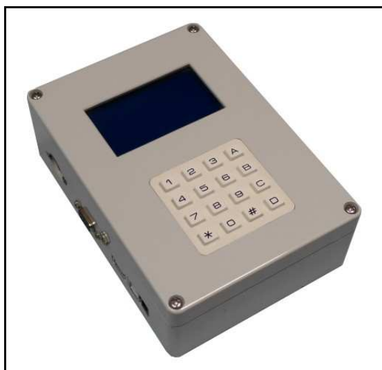
Test box fitted with monochrome graphics LCD module (128 x 64 pixels) and 4 x 4 keypad
